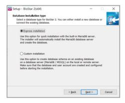
6 If Express Installation has been selected from Database Installation Type, enter the database manager's account password and click Next. If Custom Installation has been selected from Database Installation Type, enter the detailed information on the already-configured database and click Next.
